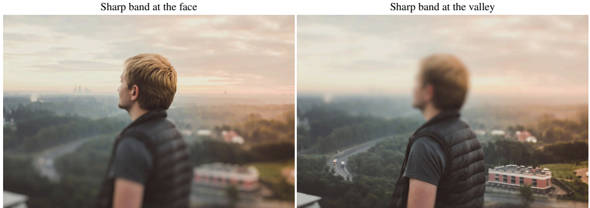
Figure H.2. Tilt-shift on a portrait. The depth given to the renderer is replaced by a vertical ramp around a chosen row, at strength K = 1 . A horizontal band stays sharp regardless of scene depth: at the face (left) the distant city and the valley blur, and at the valley (right) the buildings and the road are sharp while the subject in front blurs, giving the miniature look of a tilted lens.
